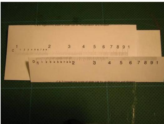
The folds in the C and D slides would now interlock to prevent separation while at the same time allowing them to slide left/right.
