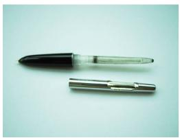
Grip the section firmly with one hand, and grip the bladder/sac protector with another. Twist and pull the bladder/sac protector.
