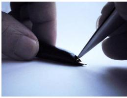
Place the tweezers in the hole and use the tweezers to pull the nib out.
